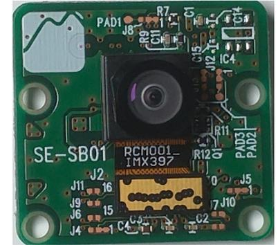
Diagonal 2.799 mm (Type 1/6.4) 0.32 Mega-Pixel (VGA) CMOS Image Sensor with Square Pixel for B/W Cameras
